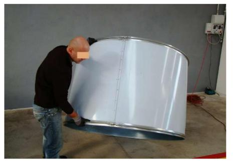
In an average assembly time of 2/3 minutes, the module (Pulsor® or DLD) is now assembled and ready to be assembled.
